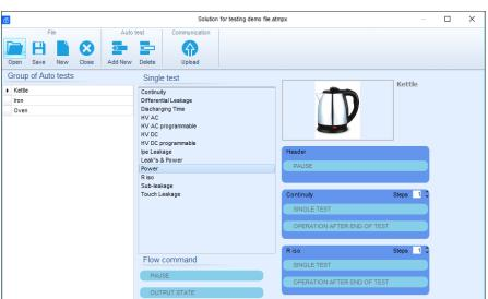
User defined structure with measurements and limits can be created on the PC SW and then uploaded to instrument.
